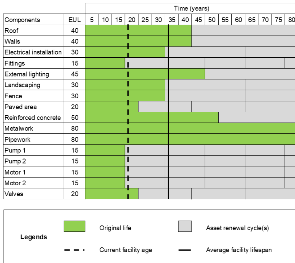
Figure 7: Timing of the replacement of the components of the pump station
